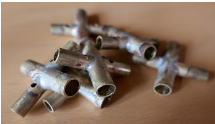
Manufacturing the 6 crosses out of brass tubes is the most time consuming part of building this antenna and will challenge your patience. The trick is to hard-solder the two pipes orthogonally together. Otherwise your Yagi antenna will look strange!
