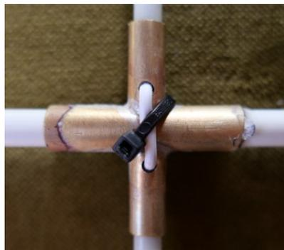
Cut wires of appx. 1 m. Feed one end through the left hole, one end through the right hole. Repeat this for all elements left. Fixate the wires with a cable tie as shown in the picture.
