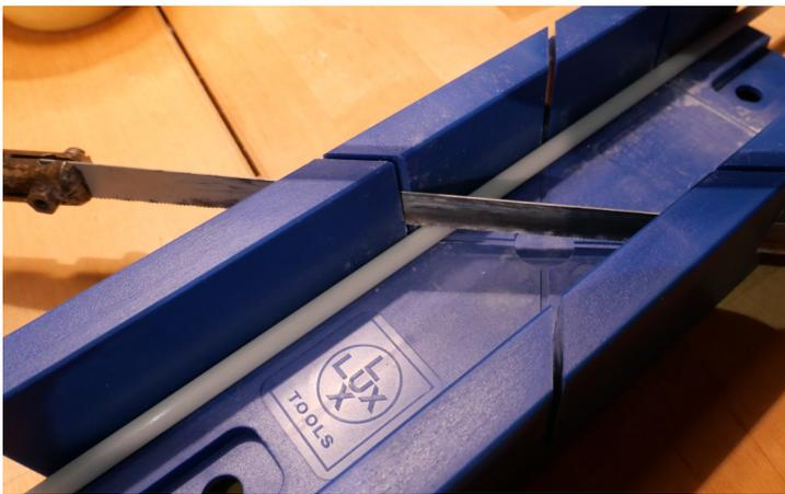
Fiberglass pipes are really a robust material, but some care has to be taken when cutting them. The ends tend to fan out. Use a hacksaw with fine teeth and a cutting jig as shown if possible. The cutting jig also helps to make the accurate 45 ° cuts in order to secure the boom against winding.
