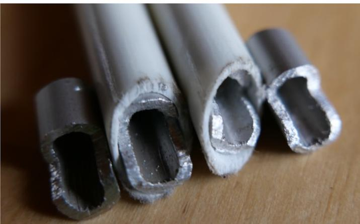
The 45 ° cuts at the boom intersections are not a perfect axial winding protection. Sometimes it needs some manual alignment by hand after setting up the antenna to make the elements being perfectly parallel. This can be improved by small inserts made of 6 mm aluminum tubes.
