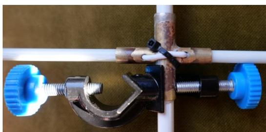
Rotating the antenna is still possible with this construction but you need to fixate the lower end of the mast construction against unwanted rotation in case of wind. This can be done by a second cross connector and a short stick which is blocked by a stone or similar.
