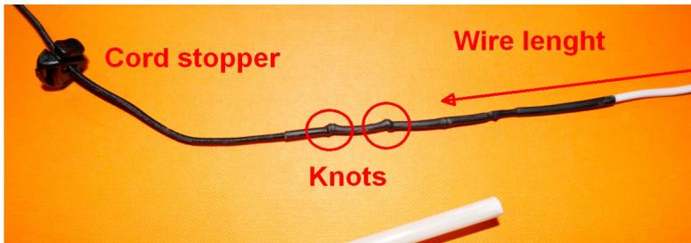
After the element wires are cut to the right length and have been fed into the brass crosses, they are connected with the 2 mm rubber cords. This is done by placing 2 small and very tight knots in the rubber cord and shrinking a 10 cm piece of 2 mm shrink tubing onto the wire and the rubber cord with the knots. The knots prevent the cord from slipping out of the shrink tubing. Rubber cord length should be around 30
