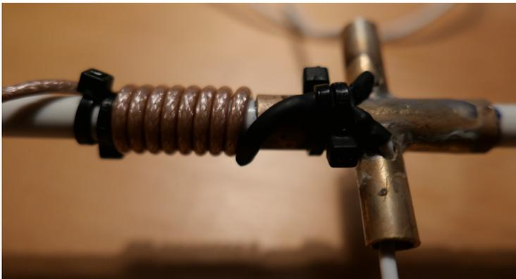
The two wires coming from the driven element have to be fed through the 3 mm holes in the brass cross as shown in the picture. Use shrink tubings to connect the wires to the RG-316 coax cable.
