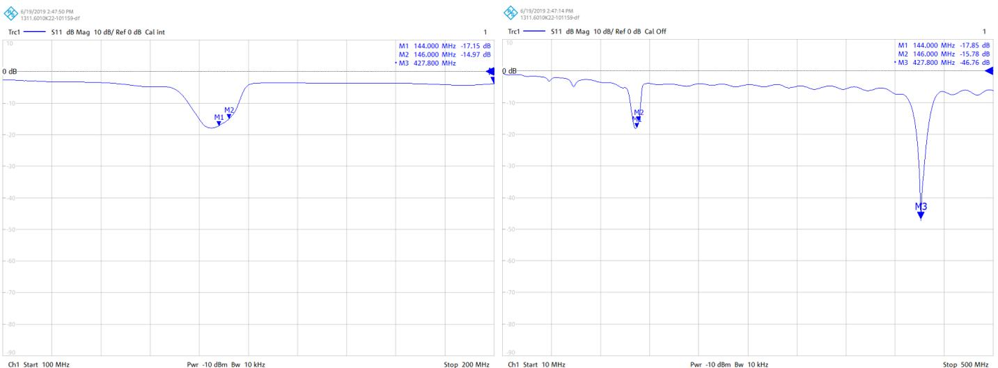
The two plots show the return loss of my second prototype antenna. I built this antenna with the element length shown in the table above which are based on simulation. Resonance is appx. 2 MHz too low but this not a real problem as the electrical design is of quite wide bandwidth.
